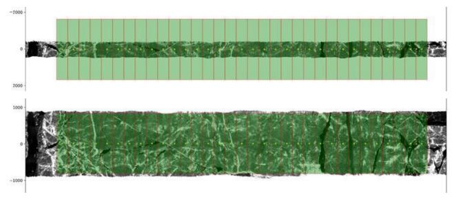
Figure 6.2: Along-track ALS surface topography with overlapping CS-2 SAR footprints. Upper plot shows ALS swath for 1 track and lower plot shows ALS surface for 5 parallel tracks covering the full width of the across-track CS-2 SAR footprints.
