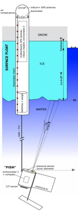
Figure 5.10: Schematic of an Ice-T buoy
