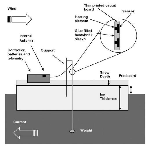
Figure 5.9: Schematic design of the SIMBA IMB setup, from Jackson et al. (2013) [RD46]
