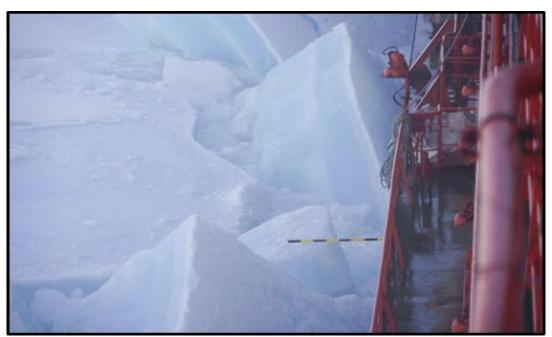
Figure 5.13: Painted pole used to aid eye in estimating ice thickness (credit: Lauren Farmer and Alex Cowen, used in Hutchings et al., 2020 [RD42]).
