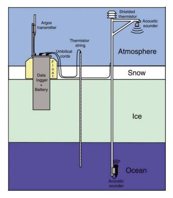
Figure 5.7: Traditional IMB schematic diagram from Polashenski et al. (2011) [RD88]
