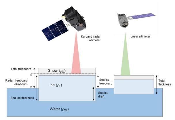
Figure 2.1: Sea ice variables and parameters of relevance to the altimetry measurements. Adapted from CPOM.
