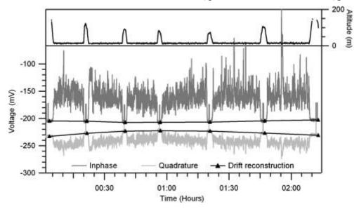
Figure 5.23 Records of Inphase and Quadrature voltages at f1 = 3.68 kHz, and flight altitude. Thick triangles mark the electrical drift determined during ascents to altitudes > 100 m above the sea surface. Note variations of high altitude measurements due to noise. Singular spikes during high altitude flights are due to calibration signals induced by calibration coils (Haas et al., 2009 [RD34]).
