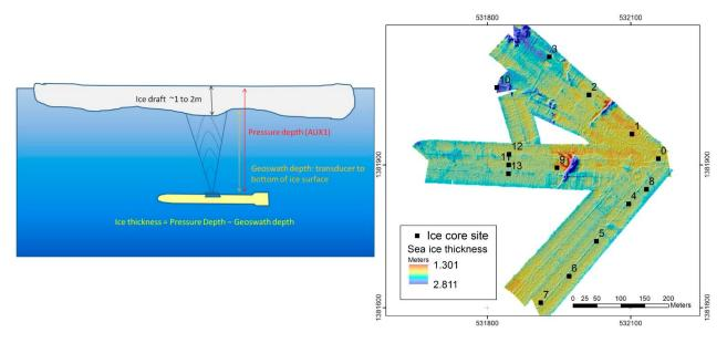
Figure 5.16: Principles of upward looking sonar mounted on AUV (left) and ice draft from survey site (right) from Lucieer et al. (2016) [RD70]
