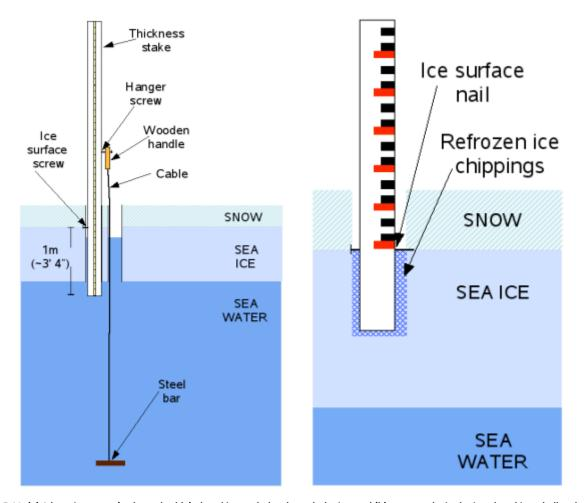
Figure 5.11: (a) A hotwire gauge (stake and cable) placed in two holes through the ice, and (b) a snow take in the ice placed in a shallow hole in the ice (Mahoney and Gearheard, 2008 [RD72]).
