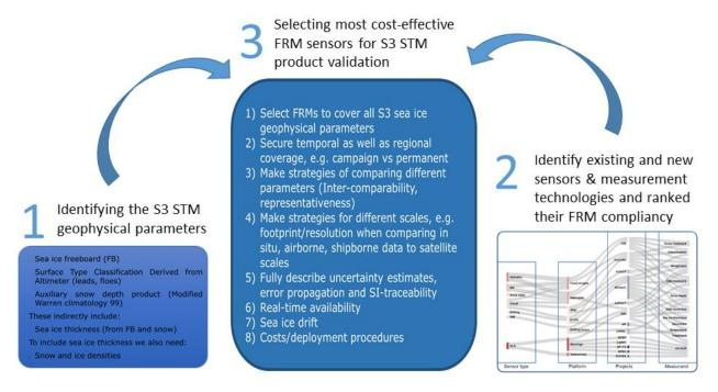
Figure 7.5: Illustration of the procedures for selecting the most cost-effective FRM for the provision of S3 STM L2 product validation. 1) S3 STM Sea ice geophysical parameters, as identified in Chapter 2, and 2) the FRM measurands based on the literature review of existing and new sensors as described in Chapter 5, together with 3) the identified steps needed in order to perform full S3 validation strategy.
