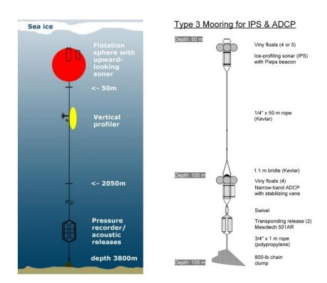
Figure 5.6: Mooring design. (a) BGEP, and (b) IOS.
