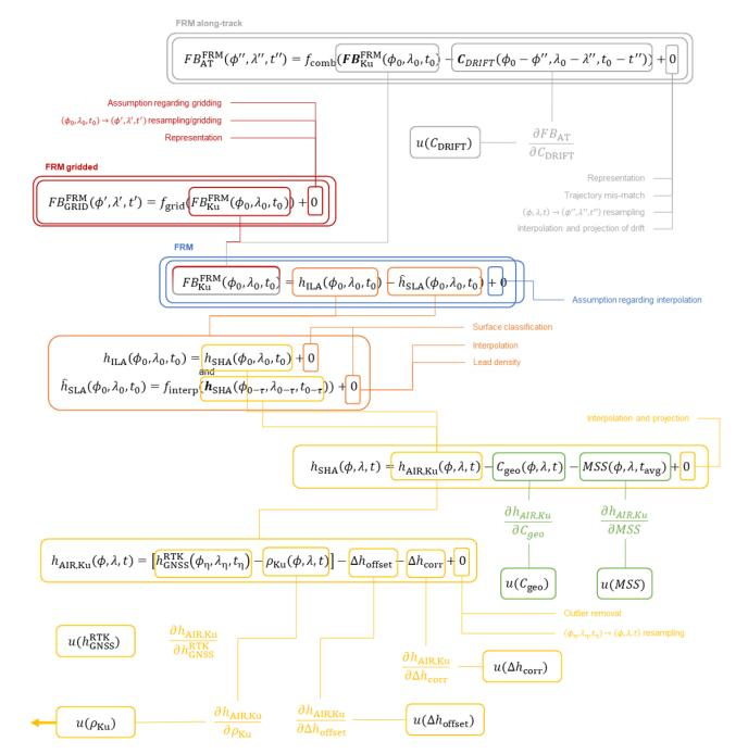
Figure 7.11 Draft example of an uncertainty traceability diagram using an airborne Ku-band radar.
