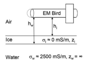
Figure 5.5: Principle of EM thickness sounding using the EM Bird, there ice thickness  $z_i$  is obtained from the difference of the bird's height above water and the ice surface ( $h_w$  and  $h_i$ , respectively).  $h_w$  is obtained with the assumption of a negligible ice conductivity  $\sigma_i$ , known water conductivity  $\sigma_w$  and horizontal layering (Haas et al., 2009 [RD34]).
