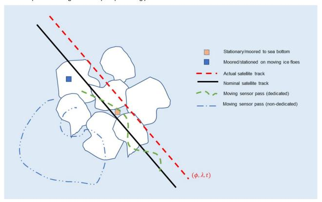
Figure 3.2: Schematic view of a generic scenario for collecting satellite altimetry and in situ data over moving/changing sea ice conditions
