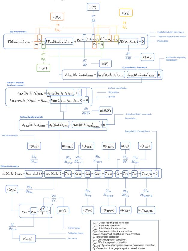
Figure 7.8: Illustration of an uncertainty diagram for sea ice altimetry and relevant measurands.
