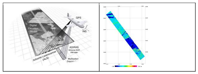
Figure 5.3: Principles of airborne swath scanner (ALS) using rotating mirrors, and ASIRAS airborne ku-band radar along a survey flight (left). Final surface topography with respect to DTU15 MSS demonstrating the high details and also the complexity of sea ice on small scales (300m x
