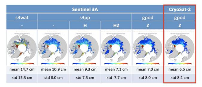
Figure 6.6: Example of comparisons between several sentinel-3A WAT freeboard products and one CryoSat-2 freeboard product (last column in the right). In the context of this project, we will consider the latest S3A LAN products.
