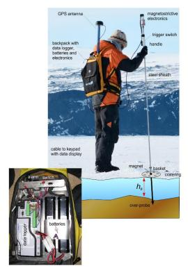
Figure 5.14: An example of a magnaprobe in use (Sturm and Holmgren, 2018 [RD105]).
