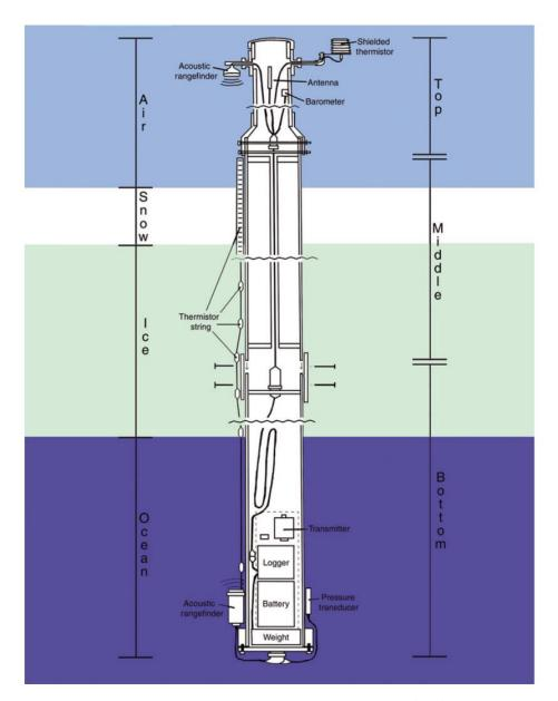
Figure 5.8: Seasonal IMB schematic diagram from Polashenski et al. (2011) [RD88]
