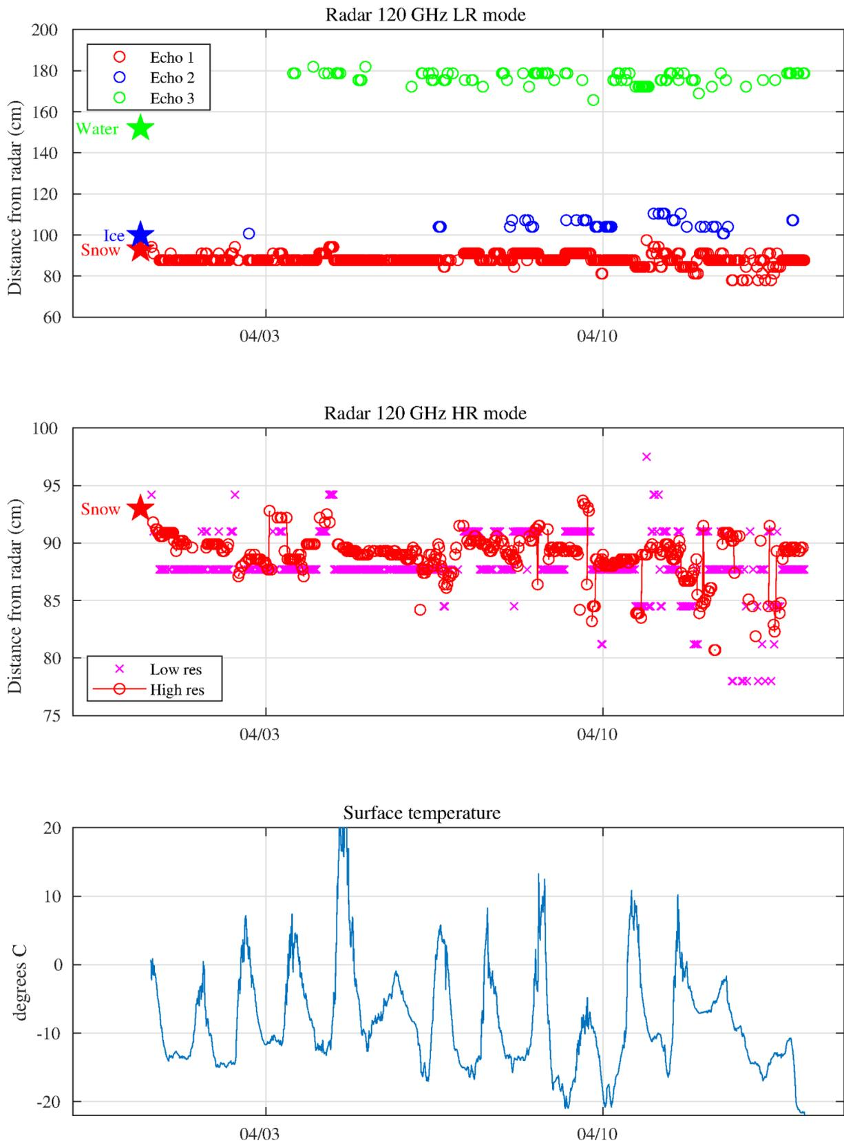
**Figure 30 - Distance to the target measured by the 120 GHz radar in LR mode (top) and HR mode (middle). Stars at the beginning of the series indicate distances to the different targets measured on the field during deployment. The evolution of the air temperature as measured by the buoy is indicated (bottom).**
