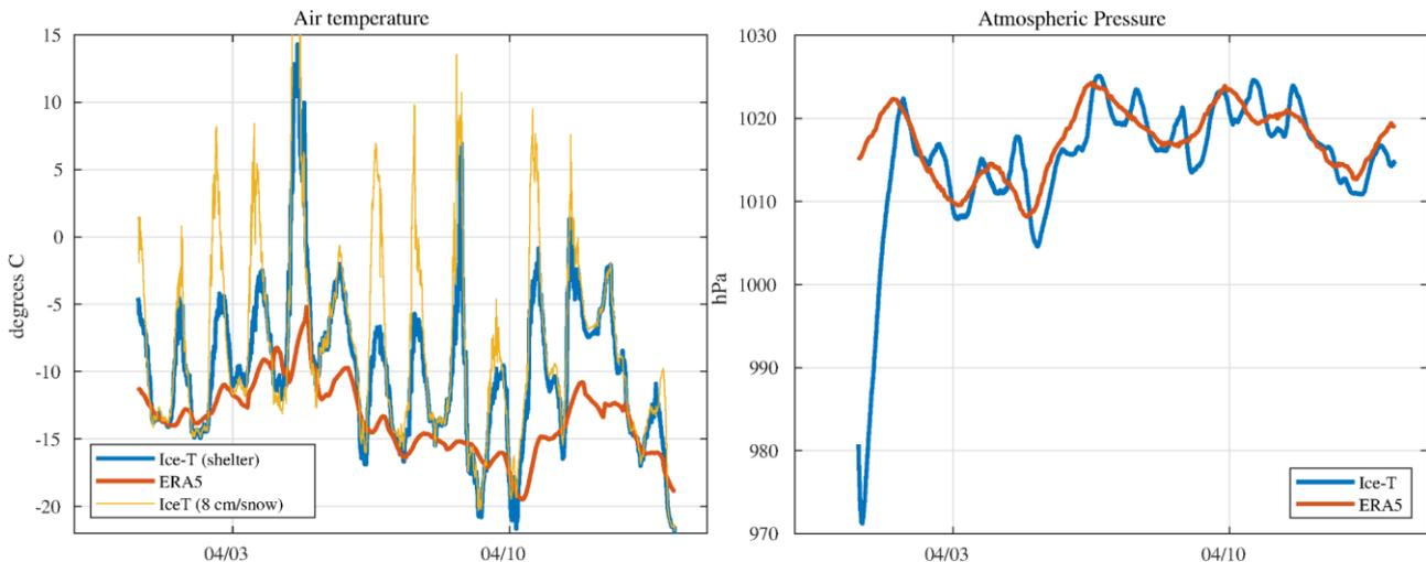
**Figure 31 - Left: Comparison of ERA5 2-m air temperature (red) with the buoy's data under its hat (shelter temperature, blue) and along the buoy 8 cm above the snow surface (yellow). Right: comparison of ERA5 and Ice-T atmospheric pressure data.**
