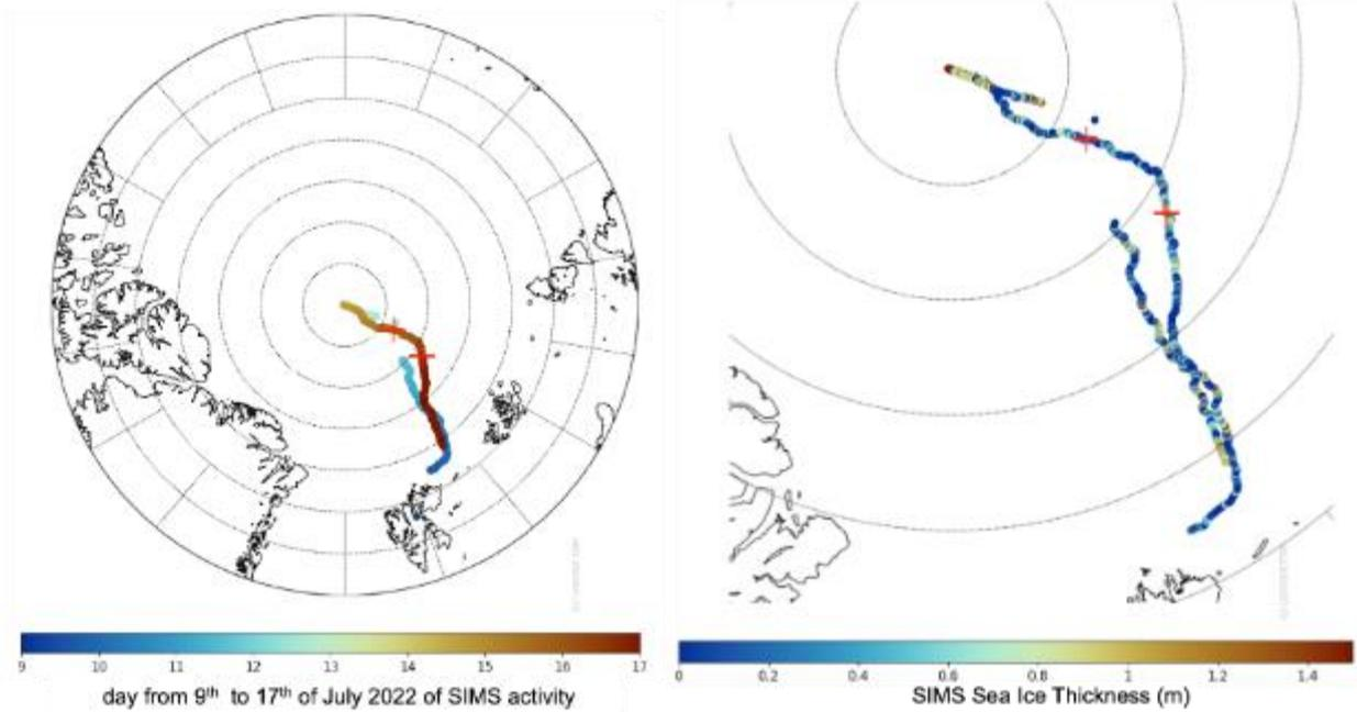
Figure 41 - The image on the left shows the trajectory of the ship recorded with the SIMS data over sea ice, the colour represents the date in day for July: the data were acquired from July 9 to 17 (with a nearly 24h of interruption from July 11 at 16:00). The image on the right shows the sea ice thickness measured by the SIMS along the trajectory. The red crosses show the places where we made freeboard measurements with the drone on the way back, once July 15th and twice July 16th.
