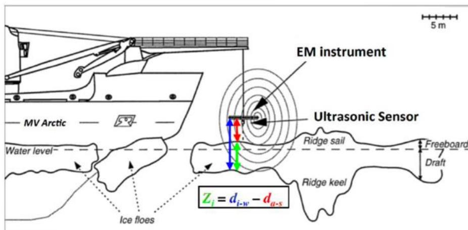
Figure 40 - SIMS measurement principle.
