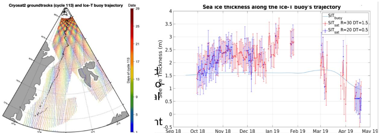
Figure 1 - Example of the Ice-T buoy trajectory and CryoSat-2 ground tracks from a cycle color-coded by the days of the cycle (left) and associated SIT comparison.
