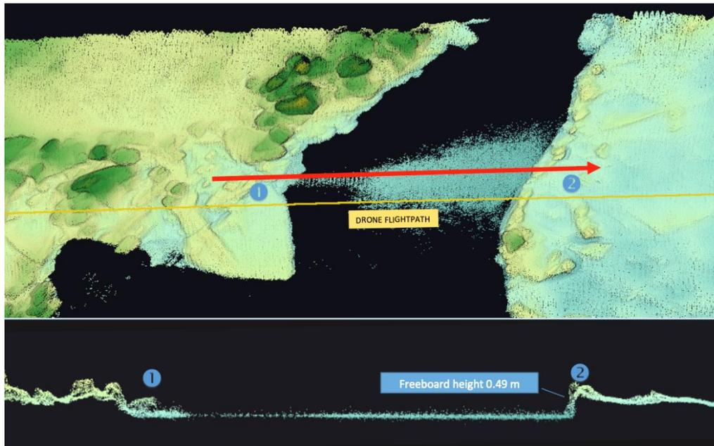
Figure 44 - A cross section over a lead between two floes. The 3D model allows to measure quite precisely a freeboard at point 2 of 49cm. The black surfaces correspond to the open water of the leads. Because of the specularity of the water only nadir shots can return back to the sensor (the points below the red arrow between the 2 floes).
