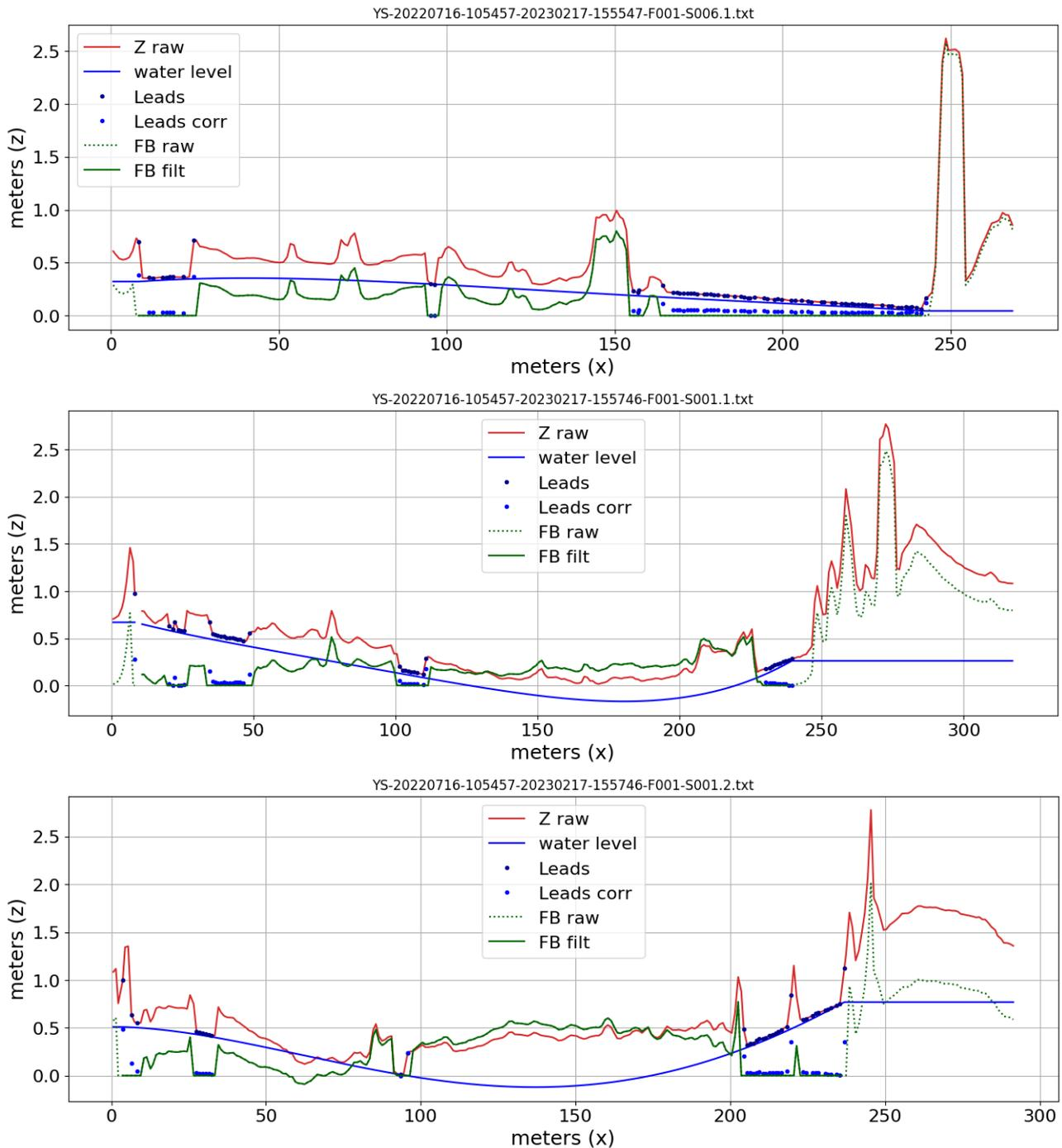
Figure 49 - The heights obtained with the YellowScan along the drone tracks are in red, with the points identified as lead measurements in blue. The blue line represents the interpolated water level that is used to correct the red height curve. The corrected curve is in green. This green curve being the height of the floes relatively to the sea level, it represents directly the freeboard of the ice
