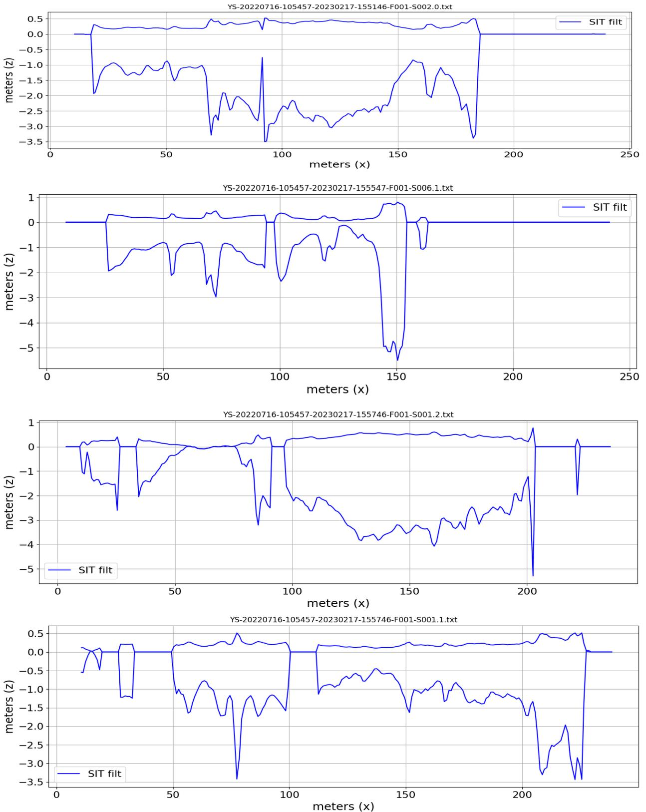
**Figure 50 – The Sea Ice Thickness is deduced from the freeboard measurement (top blue lines) and the hydrostatic equation which provides the SIT and the draft (bottom blue lines)**
