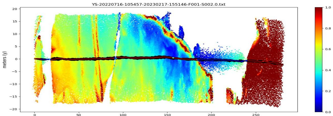
Figure 45 - A 3D scene from a top view. Only the black dots that correspond to the vertical of the drone path are kept to measure the freeboard. The colour bar represents the height of the surface in meters. The intensity of the backscatter is superimposed over these black dots.
