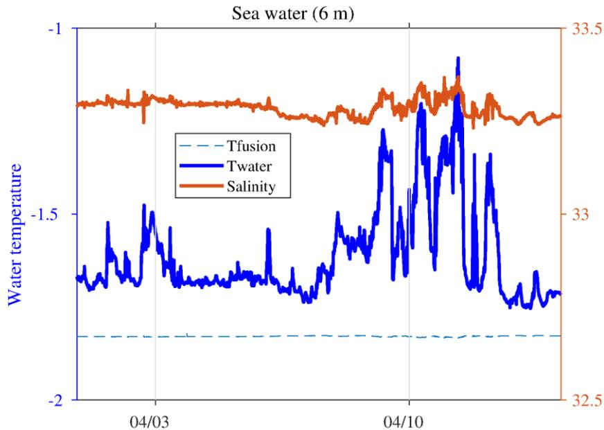
Figure 25 -Water salinity (red, scale to the right) and temperature (blue) 6m below the ice. The fusion temperature computed from in situ salinity is indicated (blue dashed line).
