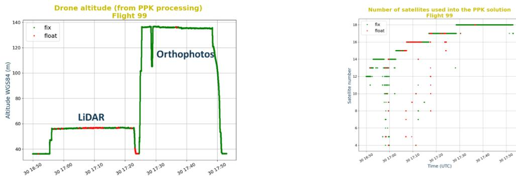
**Figure 9 - On top left, elevation of the drone embedded LiDAR altimeter during the first flight on March 30, 2022. Top right: number of GNSS satellites tracked during the first flight. Bottom left: elevation of the LiDAR altimeter during the second flight. Bottom right: number of GNSS satellites tracked during the second flight.**
