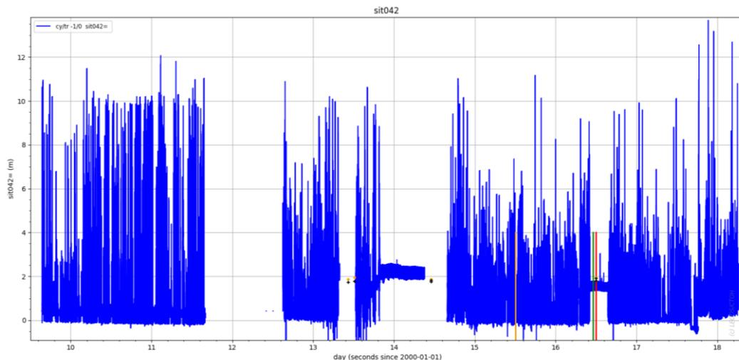
Figure 42 - Sea Ice Thickness measured by the SIMS at 1Hz. The first hole in the data around July 12th is an interruption of the SIMS (for unknown reason). The following ones correspond to stops of the ship. The more stable measurements around the 14th and end of 16th also correspond to stops of the ship over ice floes. Globally we can observe very large variations, up to 10 meters, which probably come from ridges. The 3 coloured vertical lines correspond to the drone measurements.
