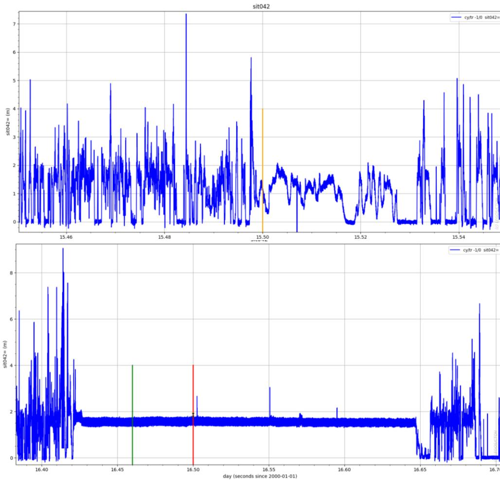
Figure 43 - Zoom of the previous Figure around July 15 at 12:00 and July 16 at 11:00 and 12:00 when we made drone measurements. Whereas some peaks reach more than 4 meters, the mean SIT value is about 1.5m to 2m. The leads can be easily distinguished with SIT=0.
