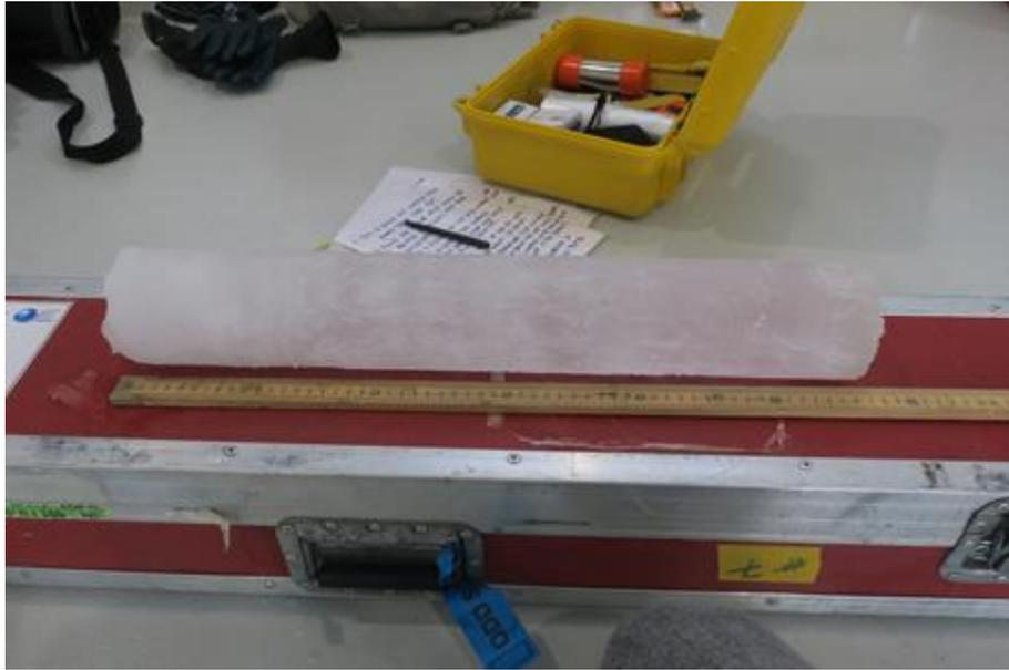
Figure 26 - 56 cm ice core collected close to the buoy during deployment on March 31, 2022
