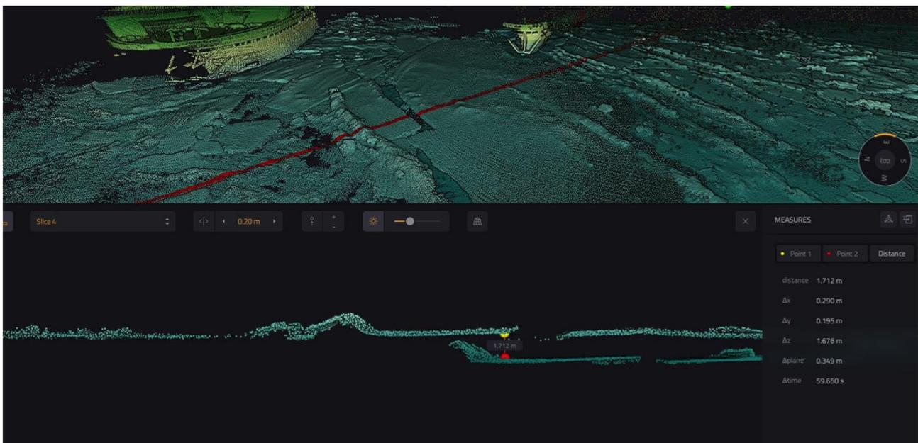
Figure 38 - A section of the previous 3D scene shows in the lower part the same floe observed by 2 successive tracks of the drone. This floe is perceived as translated of 1.75m in height between these 2 observations distant only a few tens of seconds and a few hundred meters.
