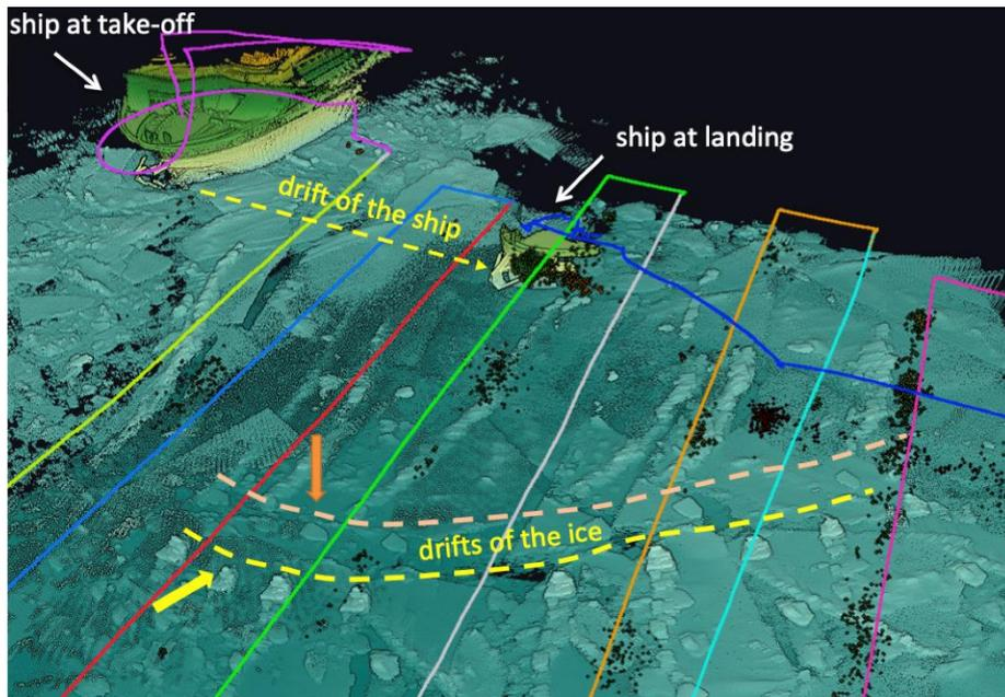
Figure 37 - A typical scene acquired with the 3D lidar scanner YellowScan during 1 flight. The colour lines represent successive paths of the drone.
