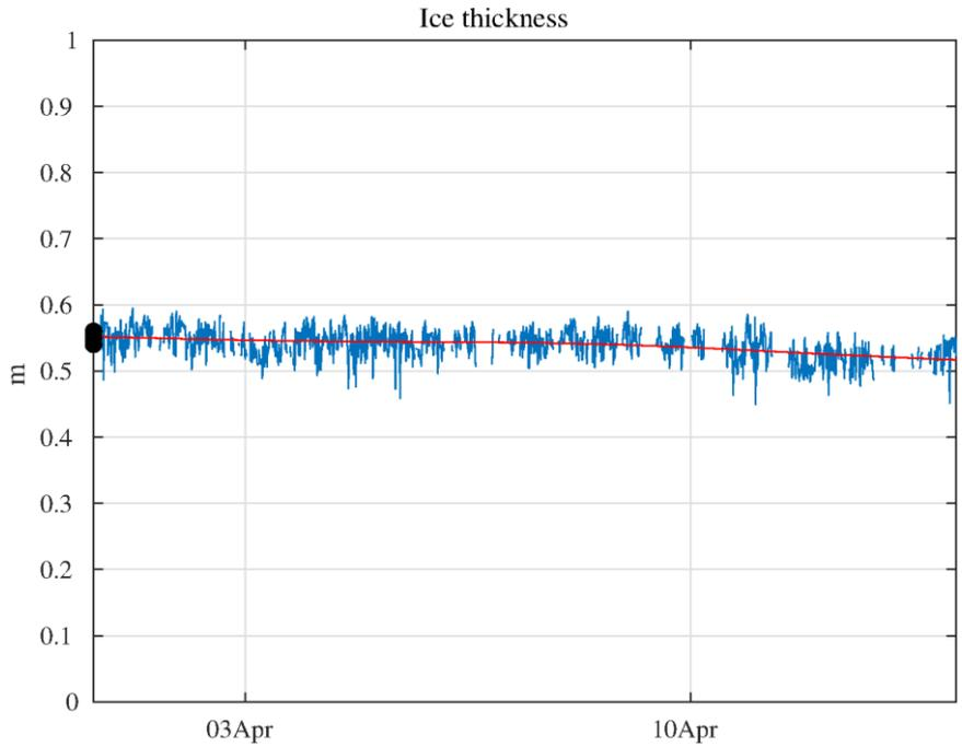
Figure 28 - Ice thickness from the Ice-T buoy (raw measurement in blue, low pass filtered in red). Black dots indicated manual soundings around the buoy at the time of deployment.
