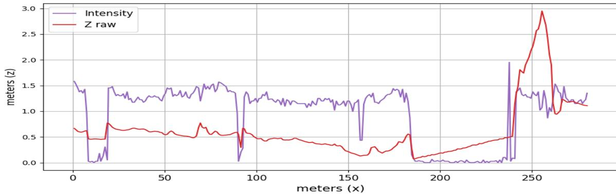
**Figure 46 - The red line corresponds to the height of the surface along the drone path shown in previous Figure 45. The purple line corresponds to the backscatter of the surface. Three leads can be easily seen which correspond to the 3 portions of minimum intensity. We can also observe that the first lead is at about 50cm height, the second tiny one at about 35cm and the large last one raise from 5cm to 50cm!**
