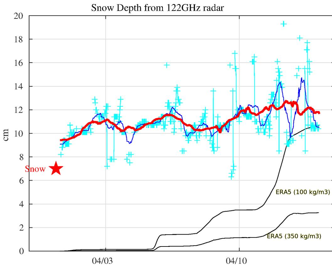
Figure 33 - Snow depth measured by the buoy (raw data in cyan, low pass filtered in red). Accumulated snowfall from ERA 5, using two values for snow density (100 and 350 kg/m<sup>3</sup>) is shown in black.
