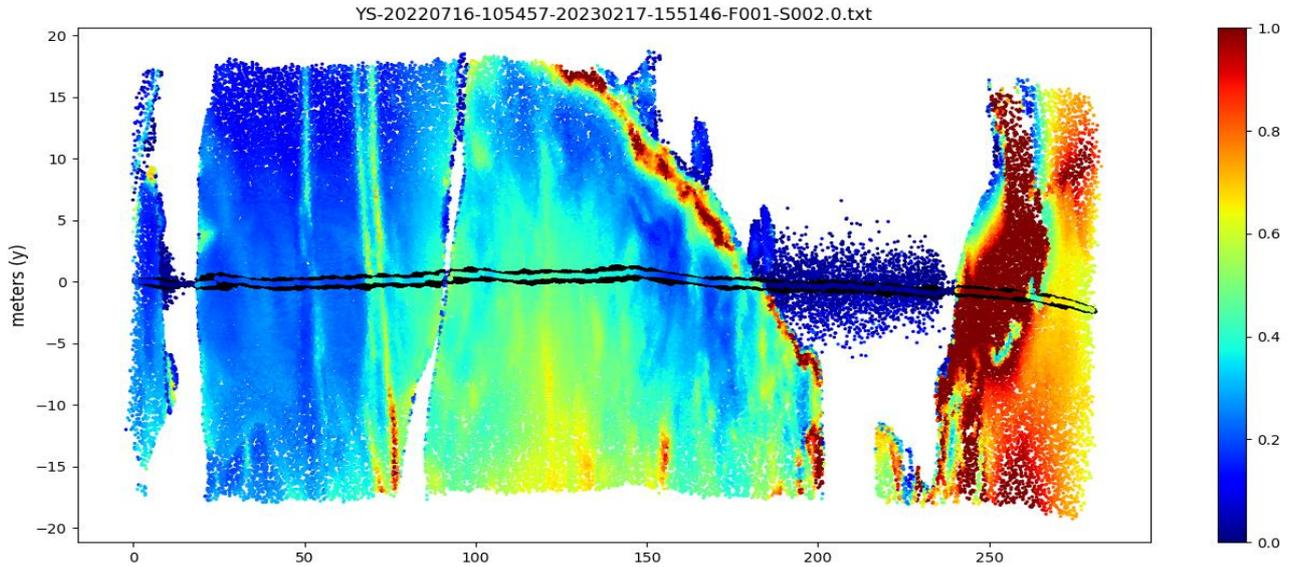
Figure 48 - The corrected height map to be compared to the original one Figure 45. The data selected to compute the correction are in black, with the height along the corrected track in colour. We observe the good continuity between the track and the measurements off-nadir.
