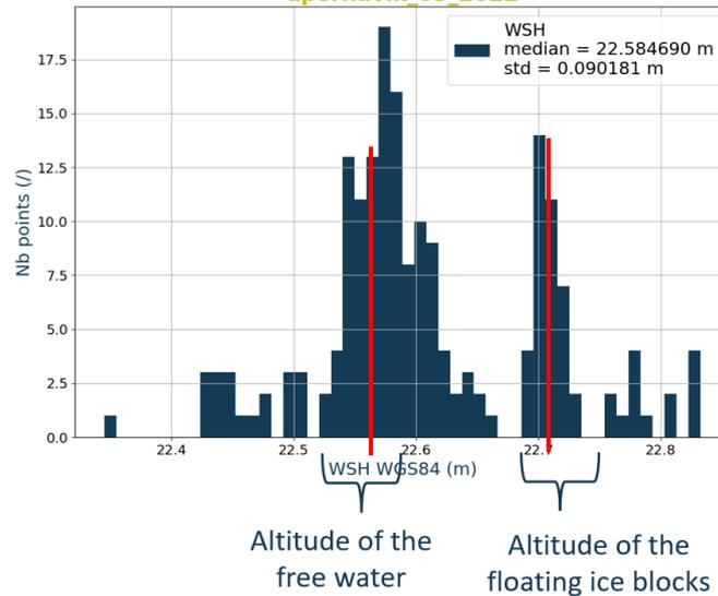
Figure 20 - Freeboard computation at the sea ice / free water interface.
