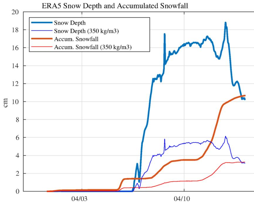
Figure 32 - ERA5 Snow Depth and Accumulated Snowfall (starting from 0) interpolated along the buoy's trajectory. Two values of snow density are used for the conversion: 100 kg/m<sup>3</sup> (ERA5 value) and 350 kg/m<sup>3</sup> (value measured on site during deployment).
