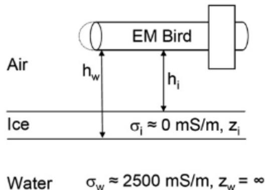
**Figure 5.5: Principle of EM thickness sounding using the EM Bird, there ice thickness  $z_i$  is obtained from the difference of the bird's height above water and the ice surface ( $h_w$  and  $h_i$ , respectively).  $h_w$  is obtained with the assumption of a negligible ice conductivity  $\sigma_i$ , known water conductivity  $\sigma_w$  and horizontal layering (Haas et al., 2009 [RD34]).**
