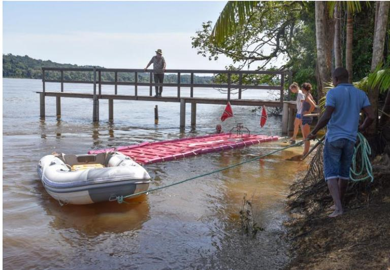
Figure 23: site 1. Showing the wharf built to support the instruments, namely a pressure sensor (in the pipe fixed to the last but one pilar), a rule (fixed to the pipe and the pilar), and the floating GNSS device (antenna being at a fixed height on the tripod) used (when trailed by a canoe) to measure the absolute level and slope of the water surface and to check for the stability of the pressure sensor (when motionless beside the wharf as it is in the picture)
