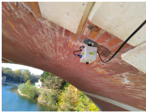
Figure 26: Picture of a vorteX.io micro-station installed on the Hers River in Mazères (South of France)
