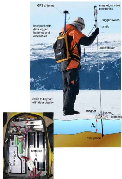
Figure 5.14: An example of a magnaprobe in use (Sturm and Holmgren, 2018 [RD104]).
