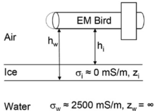
Figure 5.5: Principle of EM thickness sounding using the EM Bird, there ice thickness z_i is obtained from the difference of the bird's height above water and the ice surface ( h_w and h_i , respectively). h_w is obtained with the assumption of a negligible ice conductivity \sigma_i , known water conductivity \sigma_w and horizontal layering (Haas et al., 2009 [RD33]).
