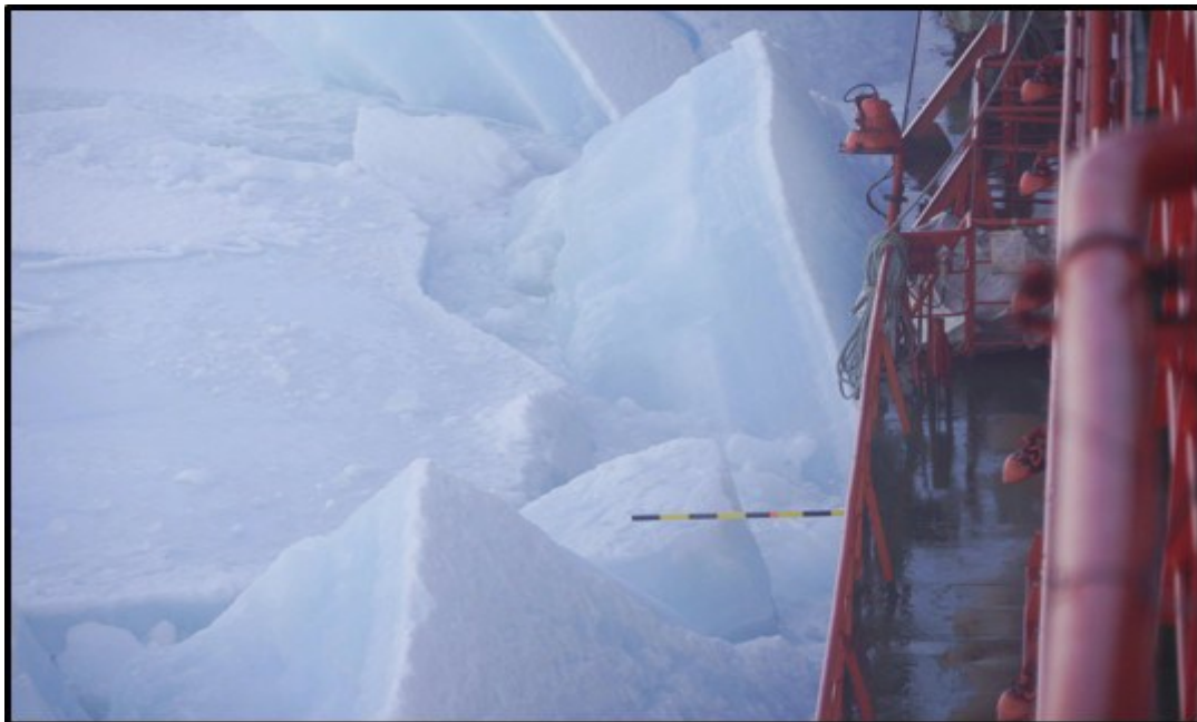
Figure 5.13: Painted pole used to aid eye in estimating ice thickness (credit: Lauren Farmer and Alex Cowen, used in Hutchings et al., 2020 [RD41]).
