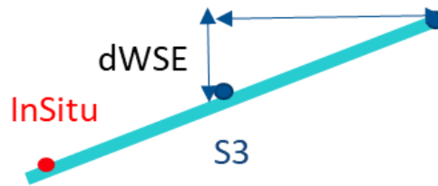
Figure 7: Scheme of the river slope impact for Cal/Val over river with a permanent in-situ sensor
