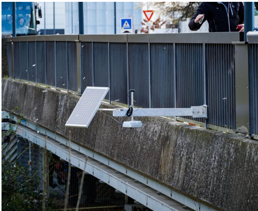
Figure 26: Picture of a V2.1 vorteX.io micro-station installed on the Hers River in Toulouse (South of France)
