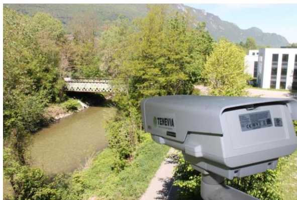
Figure 28: Example of a sensor combining a camera and a limnometric gauge
