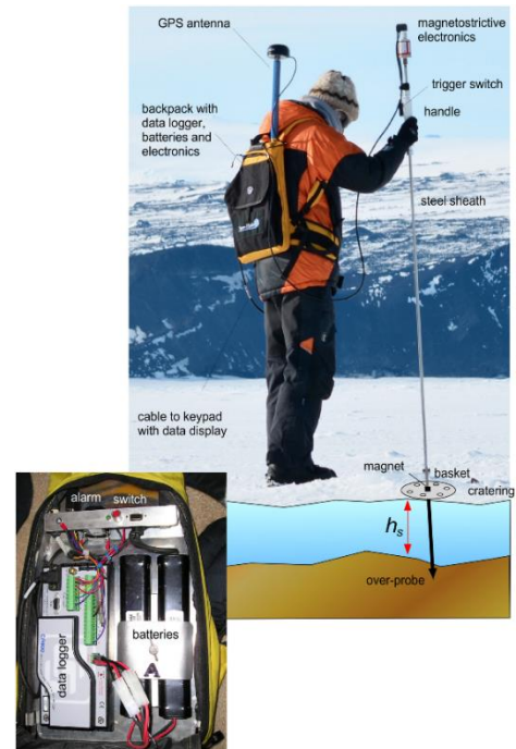
Figure 5.14: An example of a magnaprobe in use (Sturm and Holmgren, 2018 [RD104]).
