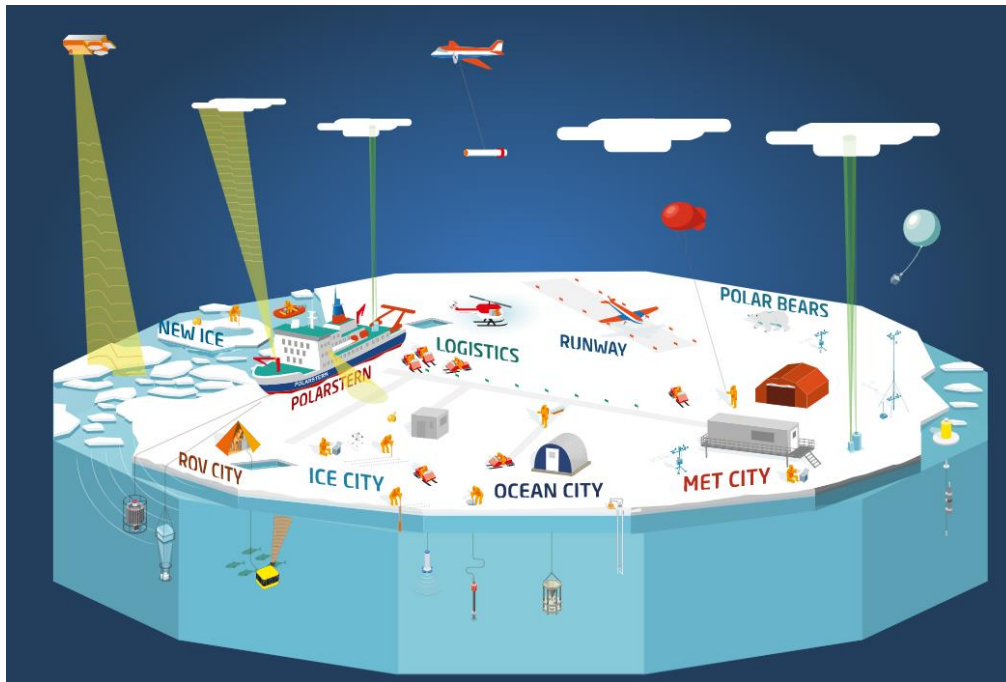
Figure 5.21: Schematic of the MOSAIC setup [RD132]
