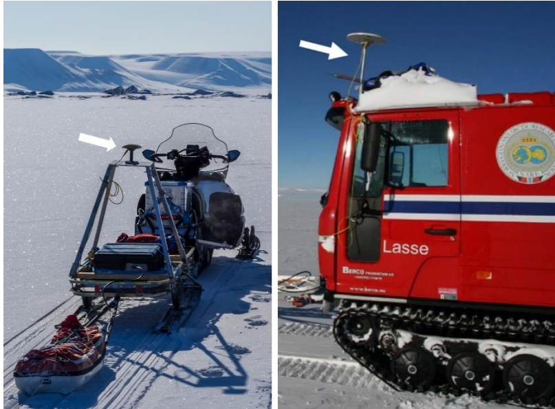
Figure 5.2 Example of geodetic GNSS mounted on a snowmobile sledge (left) and a tracked snow vehicle (right) for kinematic survey.
