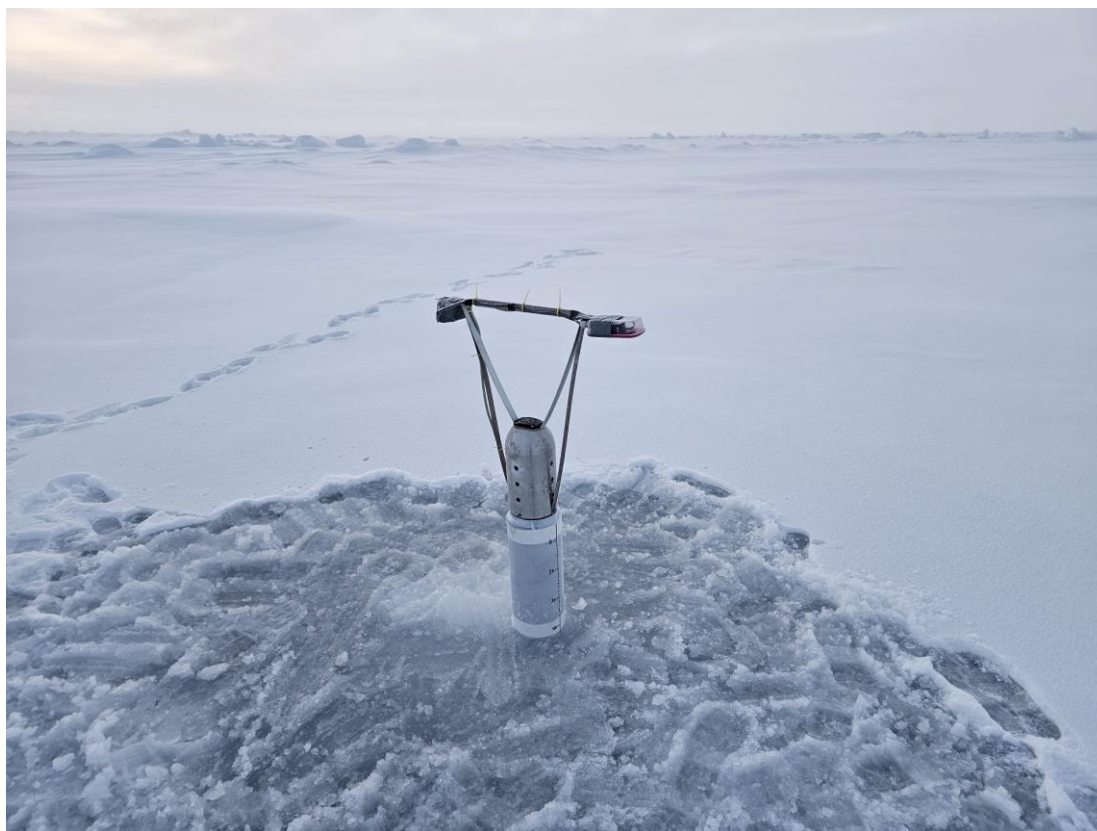
Figure 2: Ice-T buoy deployed at the Magnetic North Pole on September 16, 2025 (picture from Eric Brossier).
