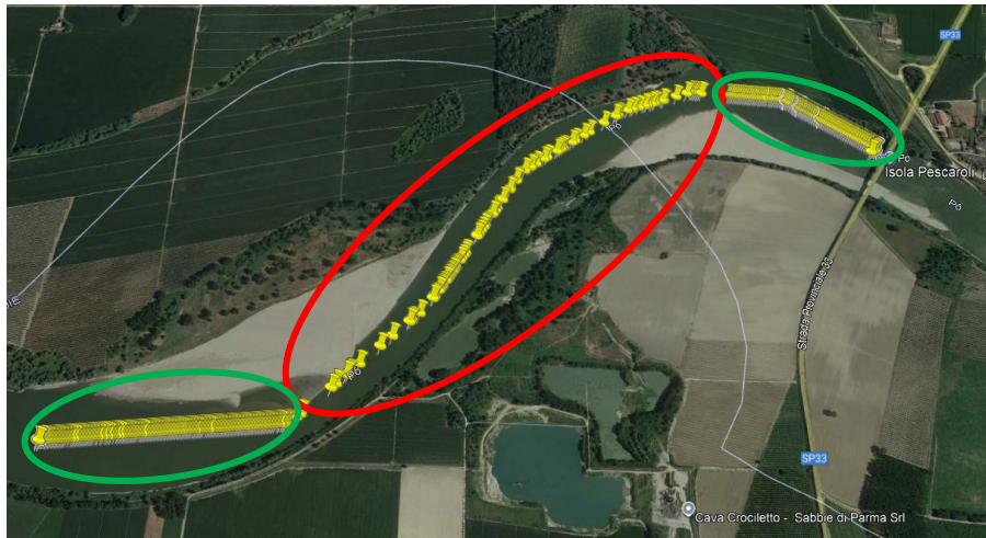
Figure 12: LiDAR measurements displayed on the map for flight 131 (in green: area without any LiDAR missing measurements; in red: area with missing measurements).
