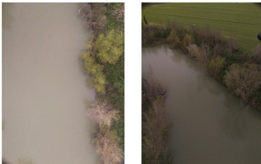
Figure 27: Pictures taken by the altimeter when the gimbal has a normal position (left) and a wrong one (right).
